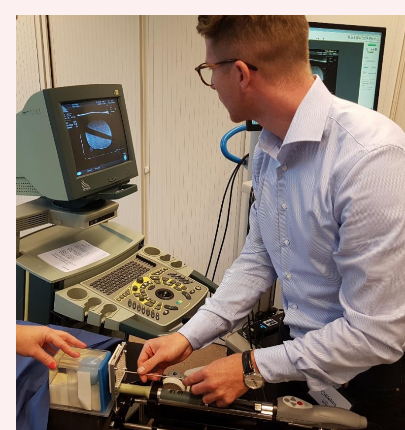
Figure 6. Testing steerable needle design
