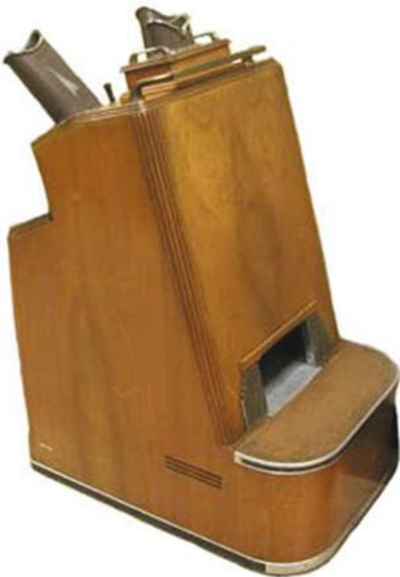
Figure 1: The Adrian machine, one of the shoe-fitting fluoroscopes. Donated by Purdue University, courtesy of Paul Ziemer.
