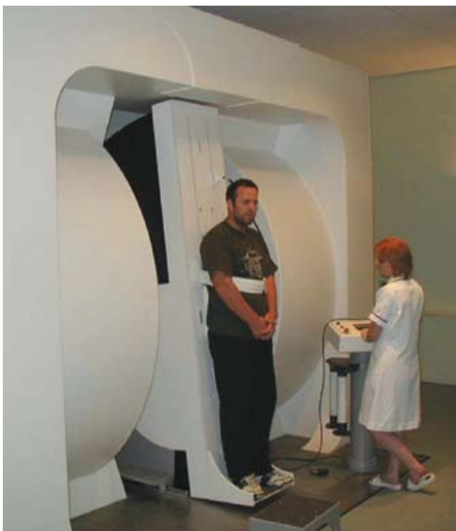
Figure 6: The 0.6 T Fonar Stand-Up MR resistive magnet (image courtesy of Frank Smith).
